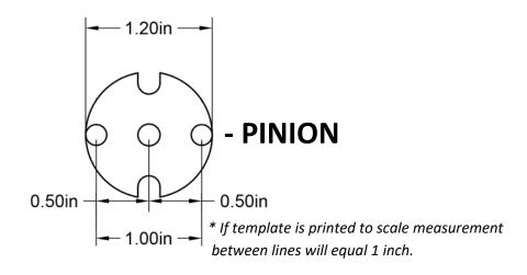
If mounting holes are required use a 7/32" drill bit for all holes.
